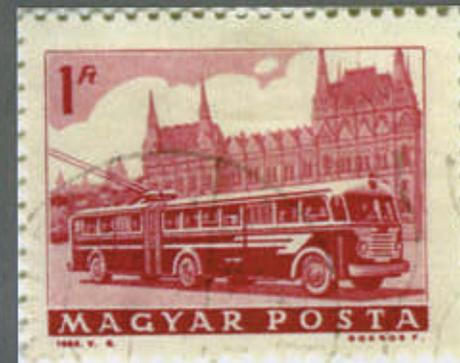
8. This Hungarian Ikarus IK-60TCS trolleybus with Ganz electrics was an interesting 1961 development of an earlier IK-60T two-axle model and was produced by adding a motorbus rear end, thus creating an articulated model. It is seen in front of the parliament building in Budapest.
